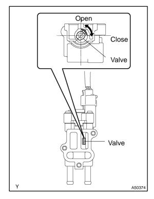
1. INSPECTION THROTTLE BODY IDLE SPEED CONTROL VALVE ASSY
