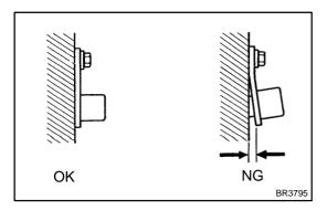
(a) Check the speed sensor installation.
