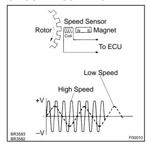
The speed sensor detects wheel speed and transmit the appropriate signals to the ECU. These signals are used for control of the ABS control system. Each of the front and rear rotors has 48 serrations.
