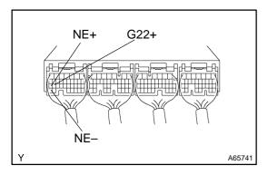
(a) Check the crankshaft position sensor for resistance.
