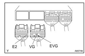
(a) Disconnect the mass air flow meter connector.
