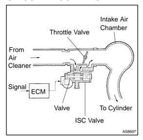
The rotary solenoid type ISC valve is located under the throttle body and intake air bypassing the throttle valve is directed to the ISC valve through the passage.
