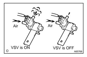
(g) Check the VSV for CCV operation when it is operated by the hand–held tester.
