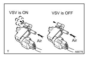
(i) Check the VSV for pressure switching valve operation when it is operated by the hand-held tester.
