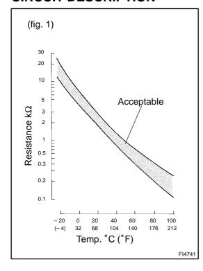
The intake air temp. sensor is built into the mass air flow meter and senses the intake air temperature.
