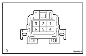
(a) Check continuity between the connector terminals shown in the chart below.
